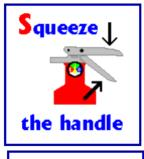
Squeeze the top handle or lever. This depresses a button that releases the pressurized extinguishing agent in the extinguisher.
